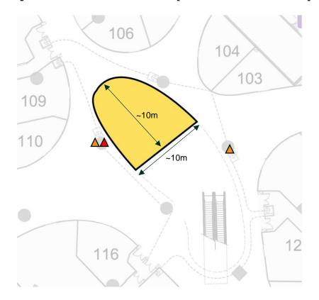
▲ 3 phase 63A power supply ▲ Single phase 13A power supply
